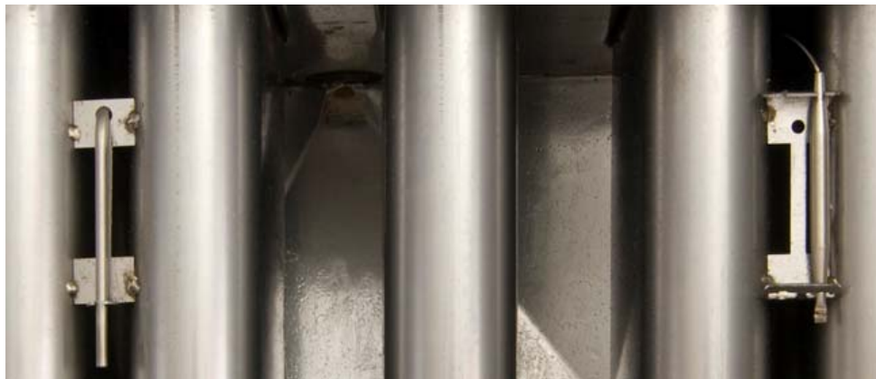
Typical sensor probe/high-limit locations and mounting hardware.
